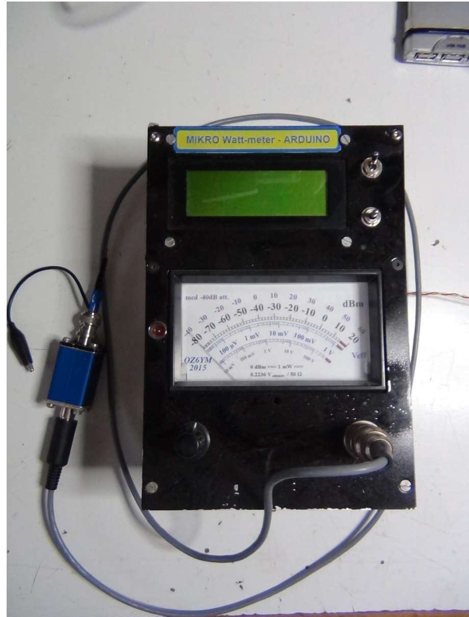
MICRO Wattmeter, 1 KHz – 500 MHz
