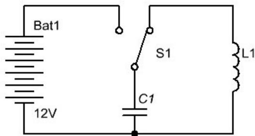
Charge the capacitor. Discharge the capacitor into the induction coil. The induction creates tension in the immediate coil environment - soft push, push, not sharp impuls. The environment pushes back causing self induction, charging the capacitor, causing consequential
